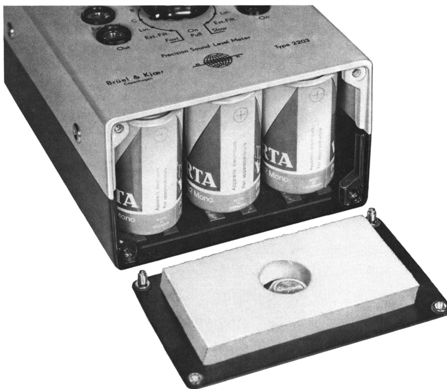
Fig.3.1. Battery compartment of 2203
